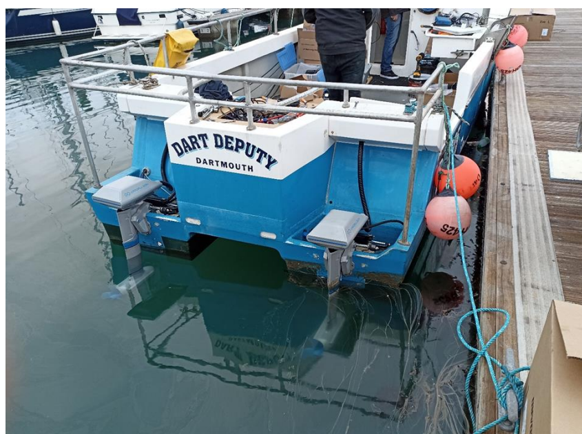
Figure 10: The “Dart Deputy”, a small potter in Devon with pure electric drive (Sergey Rybchenko).
